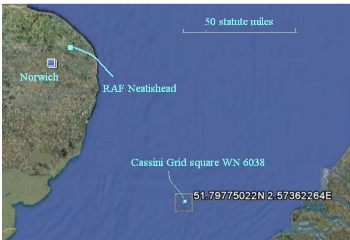
Fig.5 The small blue square indicates the 1km grid square WN6038 whose origin (SW corner) is at the lat-long coordinates shown.
