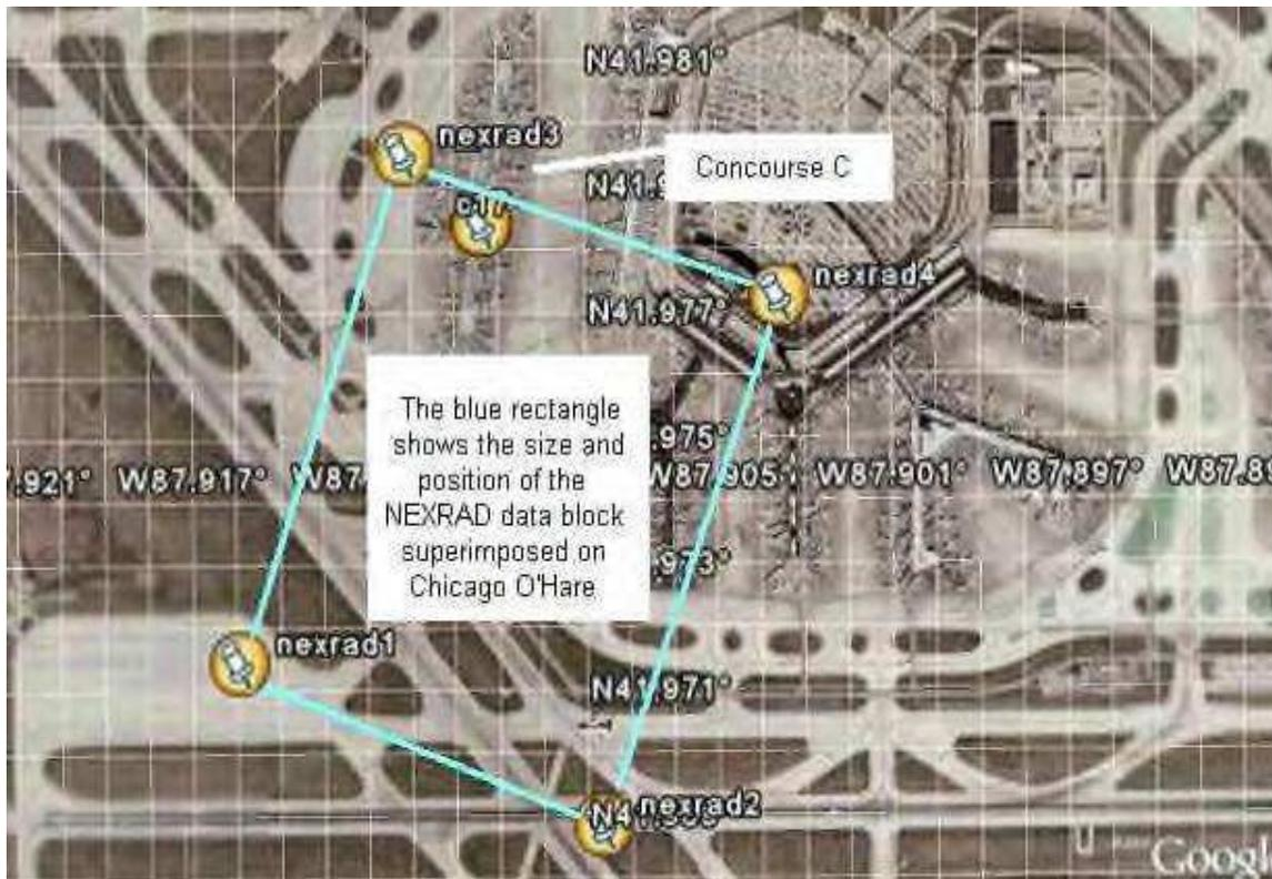
Fig.11. Showing the footprint of the NEXRAD radar resolution cell on the sighting location (adapted from image supplied by James Smith)
